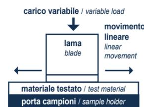
*From 2003, the shear strength of a sample taken from the glove is measured by a rotating circular blade, which moves over it in alternating directions and with constant force, until the material is completely cut. From the 2016, with the introduction of the ISO Cut Test, it is used a flat blade, which moves at a predetermined distance, subject to variable force. It was designed to better simulate an accidental cut or slash caused by a sharp object.*
